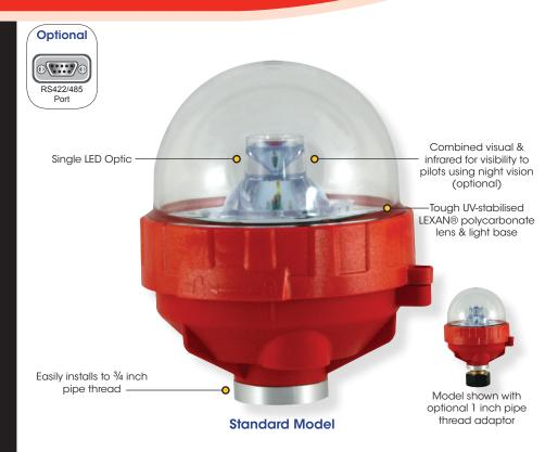
This Avlite light fixture is a steady burning, low intensity LED obstruction light designed to comply with ICAO LIOL Type A & Type B requirements. The model can be used for marking obstacles up to 45 metres above ground, such as telecommunication towers, wind turbines, buildings and other tall structures.
