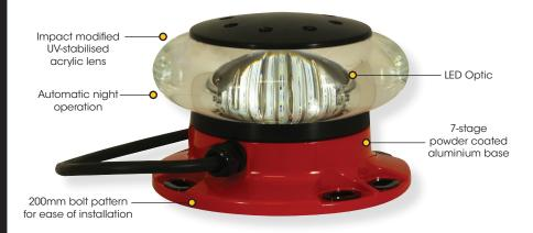
This Avlite light fixture is a flashing, medium intensity LED obstruction light designed to comply with ICAO MIOL Type B requirements. The model can be used for marking obstacles from 45-150 metres above ground, such as telecommunication towers, wind turbines, buildings and other tall structures.
