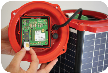
GSM module, SIM card & electronic hardware
