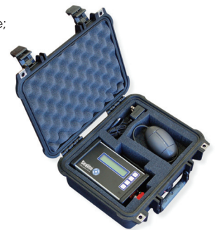
Hand-held radio controller & charger in protective case
