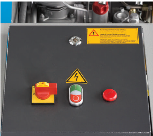
Compressor control unit of the MARINER, with main switch, on and off switches and warning light for oil level/rotation direction.
