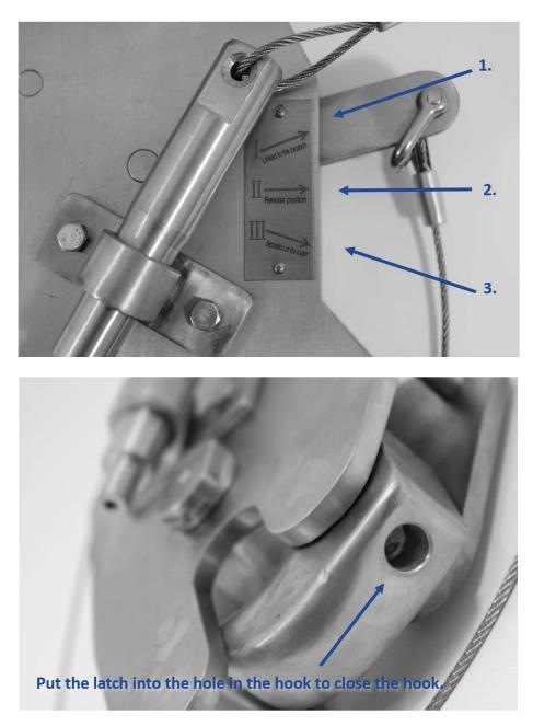
We recommend, to pull the handle and cord during lowering, just before the raft is waterborne. When waterborne, the hook will automatically open and the raft can be maneuvered away from the vessel. If a towing strain, or waves keep a load on the hook, the automatic function will not release the raft, than pull the handle/cord once more to release the hook.
