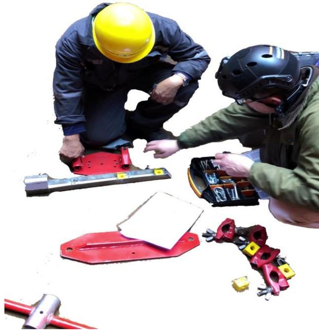
Start the assembly of Changeable High Pressure Lance Holder (Boom Head) with Rhomboid Steel Plate, SS U Profile Lance Holder.
