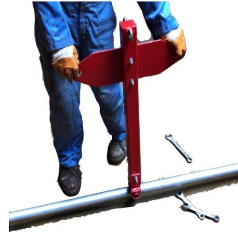
Connect the rod to the boom by using the U Shape Fixed coupler. The Steel plate should be parallel to the length of the boom.
